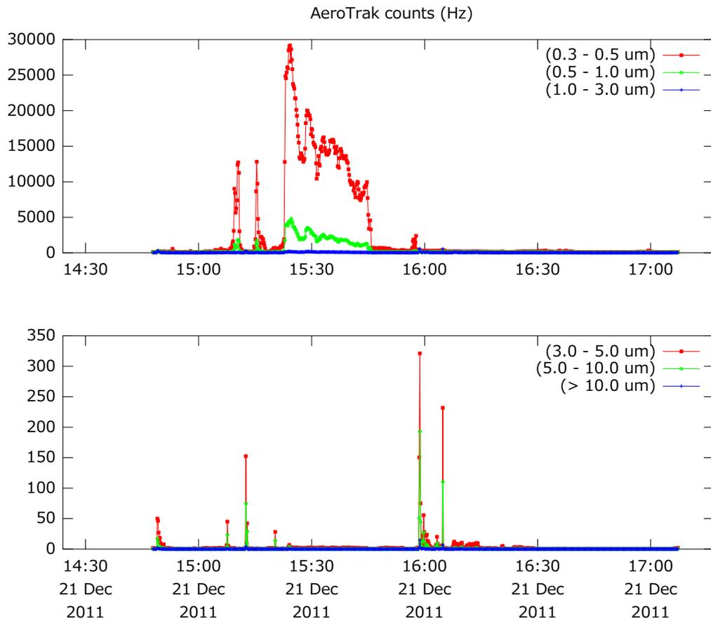
Figure 6: Time-series of AeroTrak 9306V particle counts (in Hz) versus AEST for each instrumental size channel from the mobile (car-based) survey. Top panel: Count rate for channels 1 (0.3 to 0.5  $\mu\text{m}$ ), 2 (0.5 to 1.0  $\mu\text{m}$ ), and 3 (1.0 to 3.0  $\mu\text{m}$ ). Lower panel: Count rate for channels 4 (3.0 to 5.0  $\mu\text{m}$ ), 5 (5.0 to 10.0  $\mu\text{m}$ ), and 6 (10.0  $\mu\text{m}$  and above).
