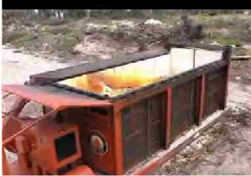
Inside the air burner
